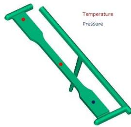
**Figure 1:** Tensile bar geometry with the locations of the pressure and temperature sensors
