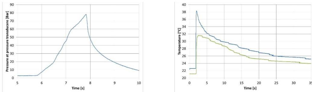
**Figure 2:** Pressure and temperature as function of time during injection with constant injection flow rate of a tensile bar geometry
